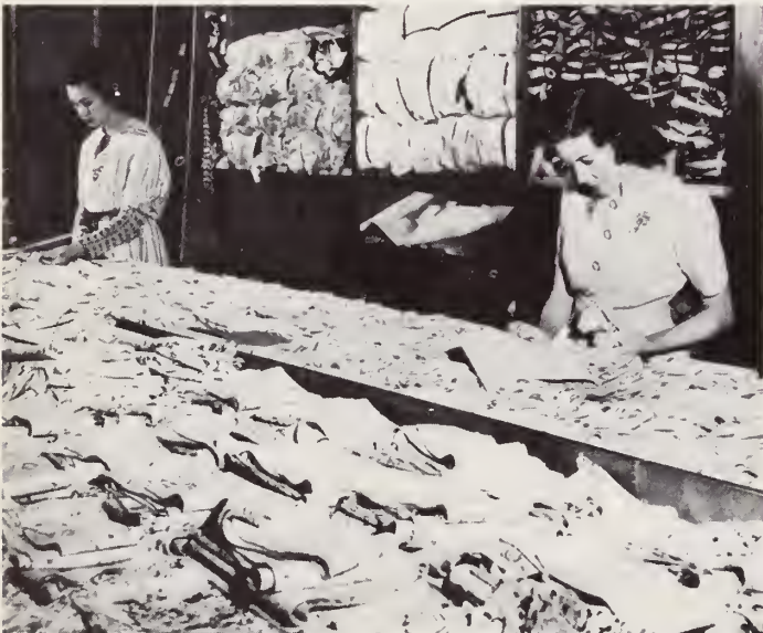
8. Assorters separate the many layers of the "lay" into "bundles" of garment parts of the same size.
