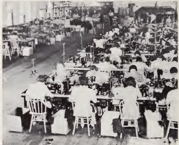
9. With treadle-controlled electric sewing machines, operators stitch together the parts of each garment.
