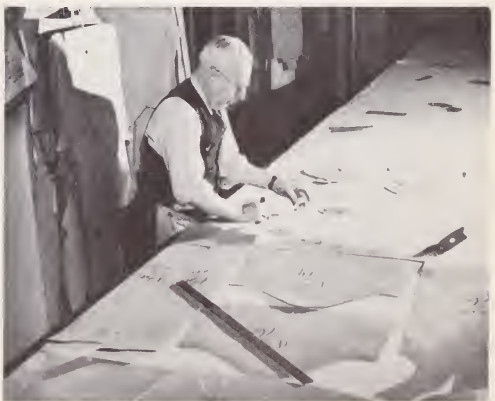
5. On a minimum yardage of fabric-wide paper, the marker traces patterns of all parts to guide cutting.
