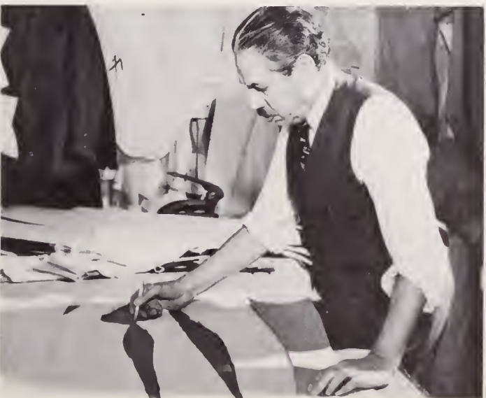
4. Sets of patterns in other sizes in the "line" are derived by grading all parts of the basic-size patterns.
