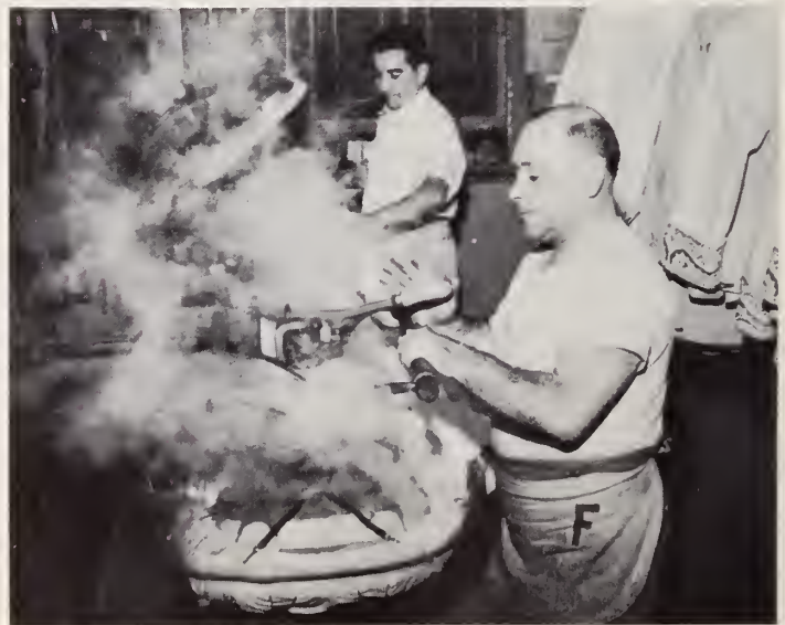
11. Creases are removed from garments with pressing machines that force live steam through the fabric.
