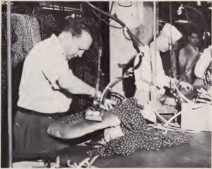
12. Seams are "opened" and smaller parts of the garment are "underpressed" with hand-controlled irons.
